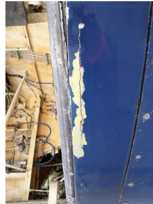
Belly fairing/wheel well panel cracked
