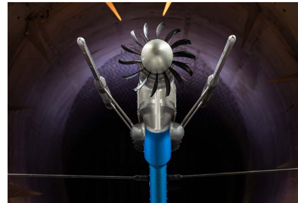
The Open Rotor, currently undergoing validation, is a disruptive propulsion architecture aiming for more efficient aviation. This ECOENGinE project (see pages 46 and 47) by Safran, supported by the DGAC and tested at ONERA in 2024, symbolizes the industry's commitment to mastering major technological challenges in aerodynamics and acoustics—crucial steps toward more sustainable propulsion. © Safran
