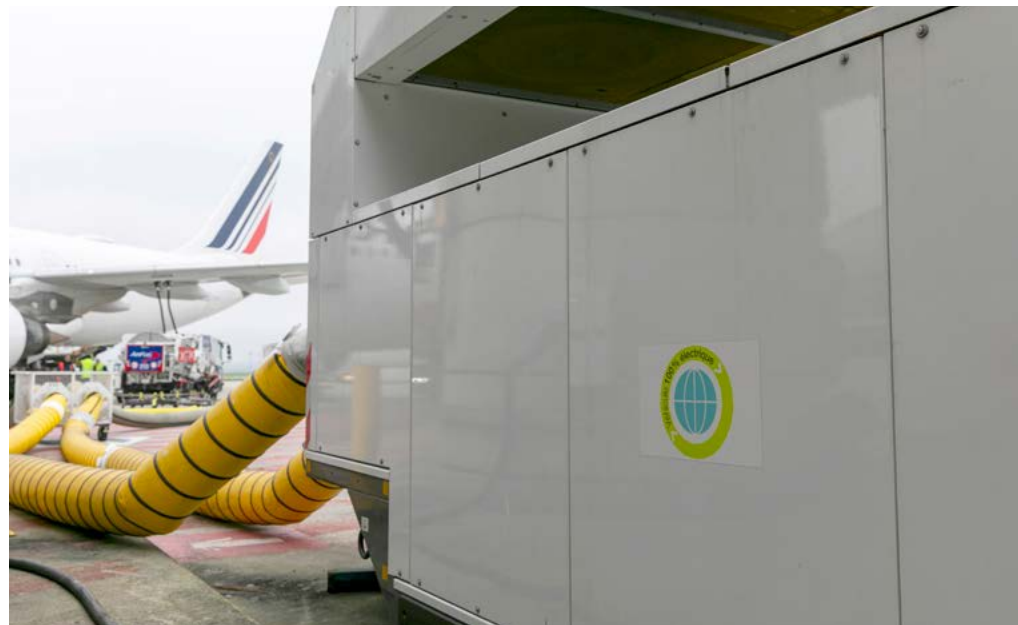
100% electric PCA air conditioning unit at Roissy-CDG airport. © Richard Metzger/DGAC-STAC
