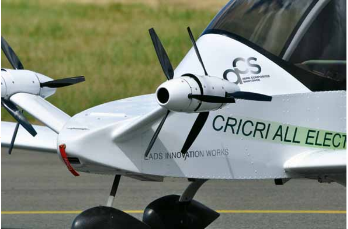
Colombar MC Cricri, 100% electric aircraft developed by EADS Innovation Works (IW), Aero Composites Saintonge and the Green Cri-cri Association
