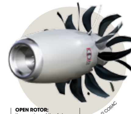
OPEN ROTOR: the engine of the future with counter-rotating high-speed propellers, from Safran.
