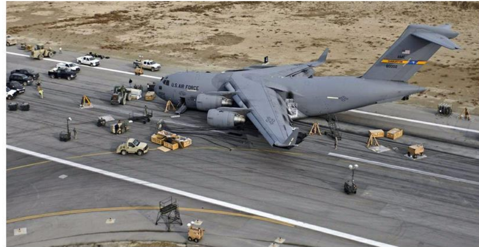
A C-17 Globemaster after a belly-landing at Bagram Airfield, Afghanistan due to pilot error (2009). Investigation pointed out aircrew distractions and task saturation
