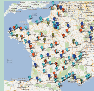
In 2016, France will offer a minimum operating network with ILS (Red) and about a hundred PBN and EGNOS procedures (Blue)
