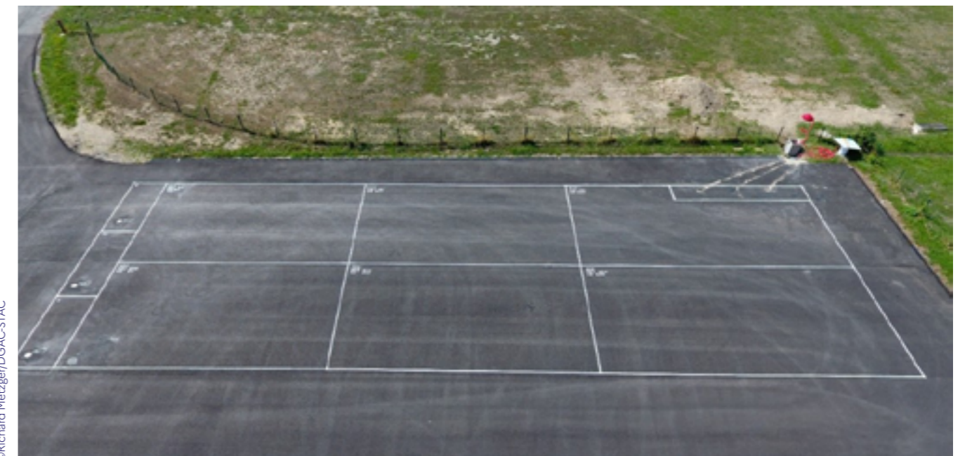
Aerial view of the experimental test strip made up of 6 sub-strips (% of different recycled aggregates)
